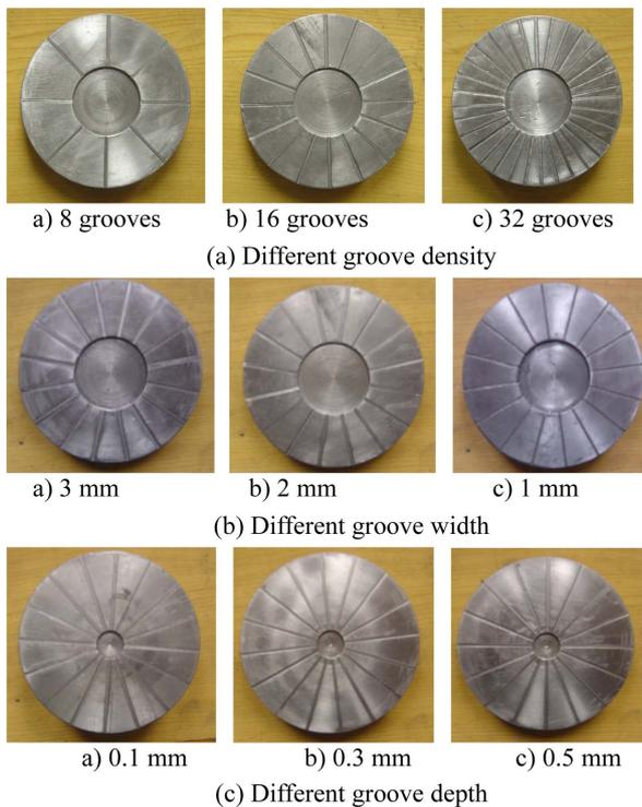
Fig. 4. (Color online) Measurement disks with different wall grooves.
