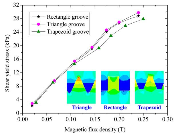
Fig. 5. (Color online) Shear yield stress of MR fluids with different groove types.
