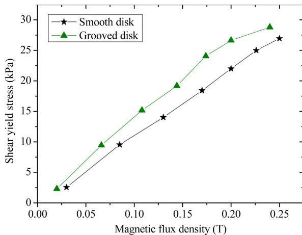
**Fig. 9.** (Color online) Shear yield stress obtained by smooth disk and grooved disk.
