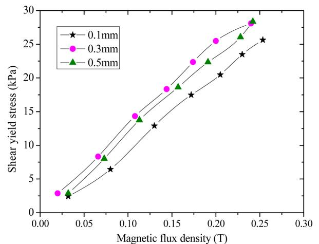
**Fig. 8.** (Color online) Influence of radial groove depth on shear yield stress.
