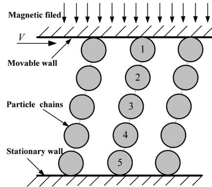
Fig. 2. Relationship between particles and wall.
