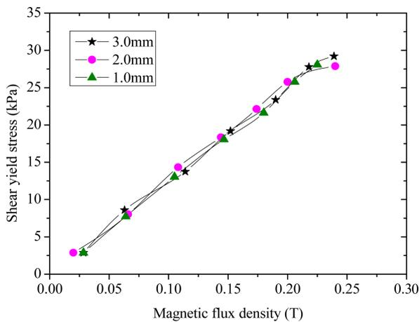
**Fig. 7.** (Color online) Shear yield stress of MR fluids with different groove depths.
