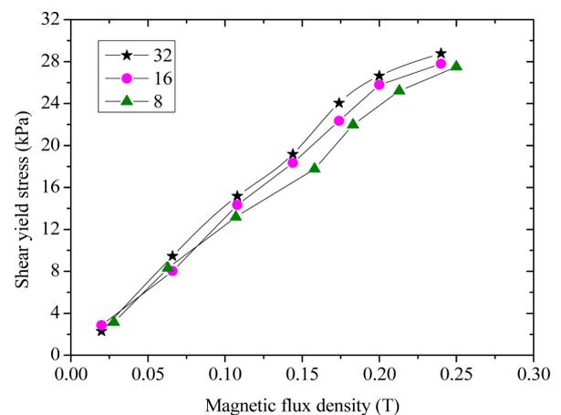
Fig. 6. (Color online) Shear yield stress of MR fluids with different groove densities.
