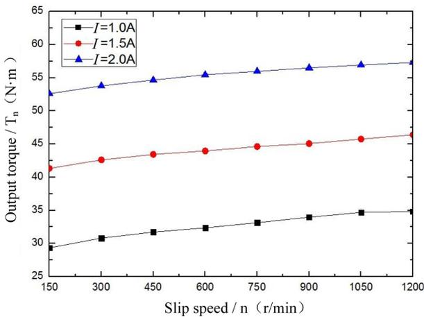
**Fig. 11.** (Color online) Relationship between output torque and slip speed.
