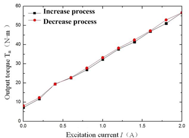
Fig. 10. (Color online) Relationship between output torque and excitation current.
