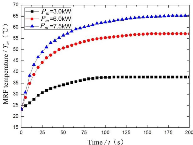
**Fig. 13.** (Color online) Temperature variation curves of MRF under different slip powers (Water-cooling state).
