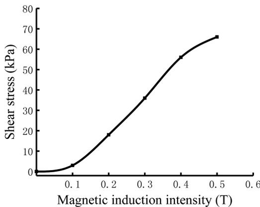
Fig. 8. Shear stress of the chosen MR fluid.
