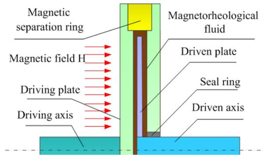
Fig. 2. (Color online) Structure diagram of transmission unit.
