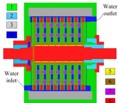
Fig. 4. (Color online) 3D simplified model of temperature field.
