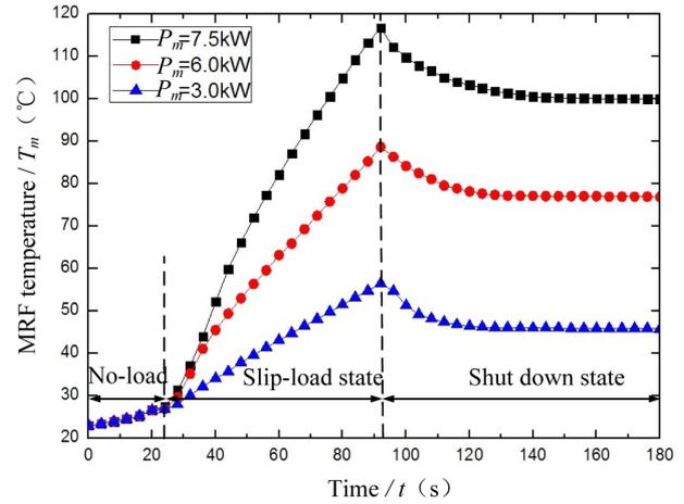
**Fig. 12.** (Color online) Temperature variation curves of MRF under different slip powers (Natural-cooling state).
