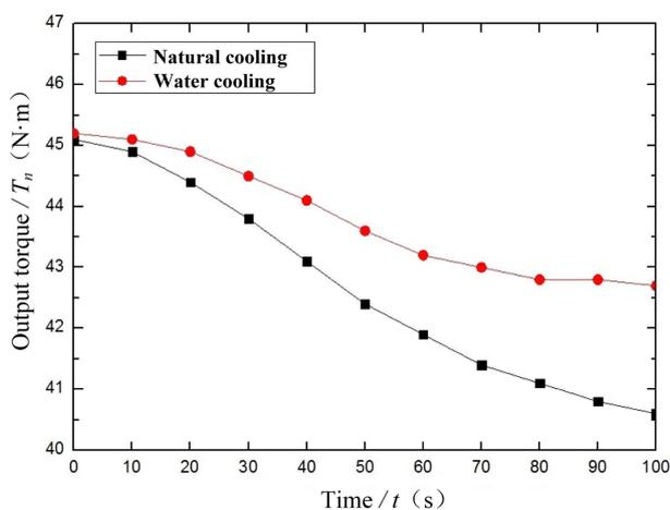
**Fig. 14.** (Color online) Variation curves of output torque under different cooling conditions.
