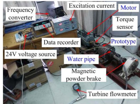
Fig. 9. (Color online) Photograph of test-bed system.
