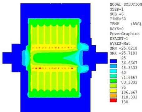
**Fig. 5.** (Color online) Temperature distribution of water-cooling MRTD with natural cooling.
