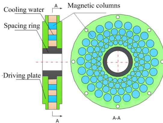
Fig. 3. (Color online) Structure diagram of cooling unit.
