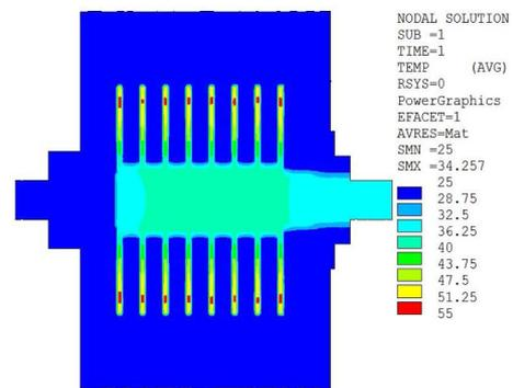
**Fig. 6.** (Color online) Temperature distribution of water-cooling MRTD with water cooling.
