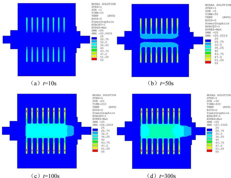
**Fig. 7.** (Color online) Temperature distribution of water-cooling MRTD with different times.
