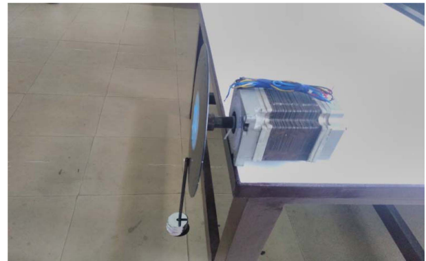
Fig. 29. (Color online) Experimental setup for measuring cogging torque.
