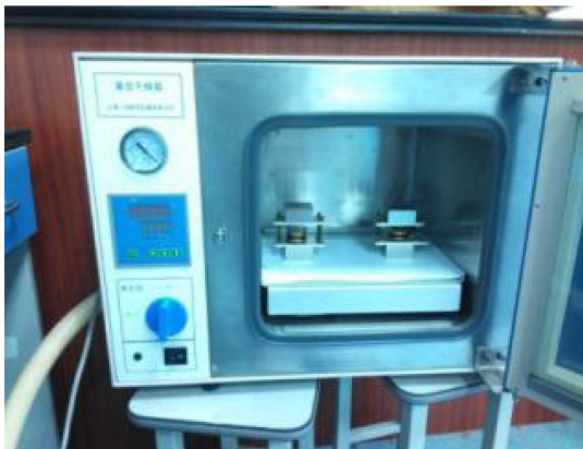
Fig. 5. (Color online) Base material curing device.
