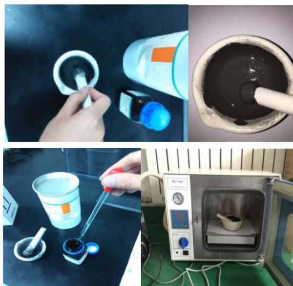
Fig. 3. (Color online) Mixing and grinding, add curing agent and vacuum.
