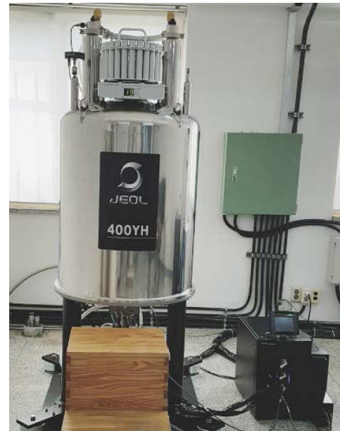
Fig. 1. (Color online) 400 MHz FT-NMR spectrometer used in this study.
