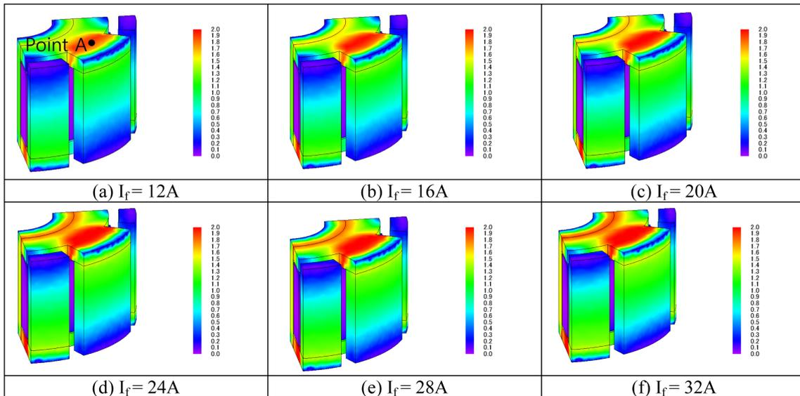
Fig. 2. (Color online) Flux density of rotor core.
