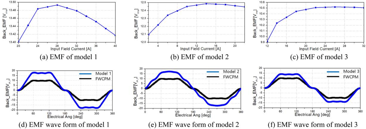
**Fig. 6.** (Color online) No-load characteristics of the FAFWCPM.
