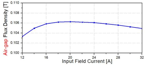
(b) Air-gap flux density based on field current
