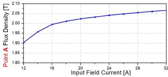
(a) Point A flux density based on field current
