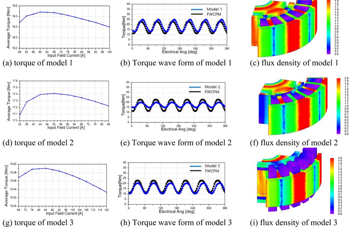
**Fig. 7.** (Color online) Load characteristics of FAFWCPM.
