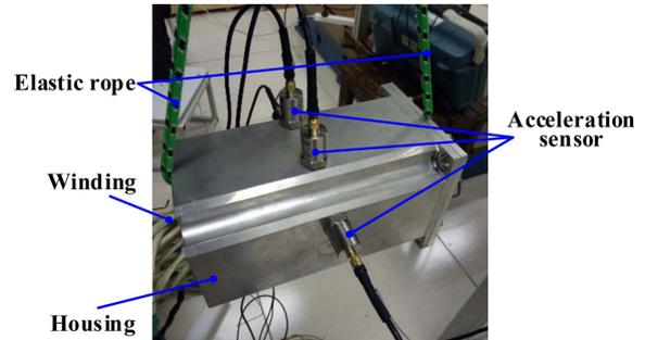
**Fig. 15.** (Color online) Modal experiment of prototype.
