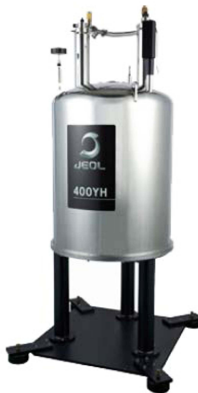
Fig. 1. (Color online) FT-NMR 400 MHz Spectrometer used in the total fluorine content of fluoride toothpaste.
