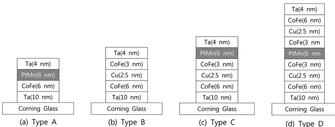
**Fig. 1.** Schematic structure of one CoFe/PtMn bilayer ((a) Type A) and three different types ((b) Type B, (c) Type C, and (d) Type D) of CoFe/Cu/CoFe SV multilayer without or with antiferromagnetic PtMn layer.
