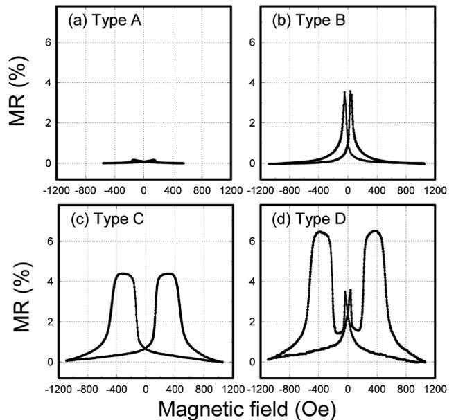
**Fig. 3.** Major MR curves according to the easy axis for four types ((a) Type A, (b) Type B, (c) Type C, and (d) Type D) after post-annealing treatment.
