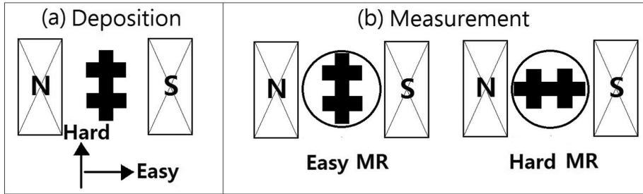
**Fig. 2.** Schematic of the easy and hard axis direction for the applied magnetic field under (a) multilayer deposition and post-annealing treatment, and (b) MR measurement.
