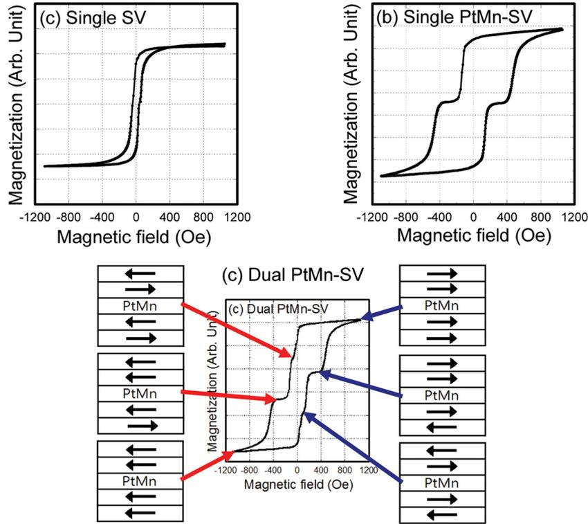
**Fig. 5.** (Color online) Two different MH loops for (a) the spin valve multilayer and (b) the single-type GMR-SV multilayer with PtMn corresponding to integrated MH loop for (c) the dual-type CoFe/Cu/CoFe/PtMn/CoFe/Cu/CoFe GMR-SV multilayer. Arrows of inset in Fig. 5(d) are the spin configuration of each ferromagnetic layer in dual-type PtMn GMR-SV multilayer.
