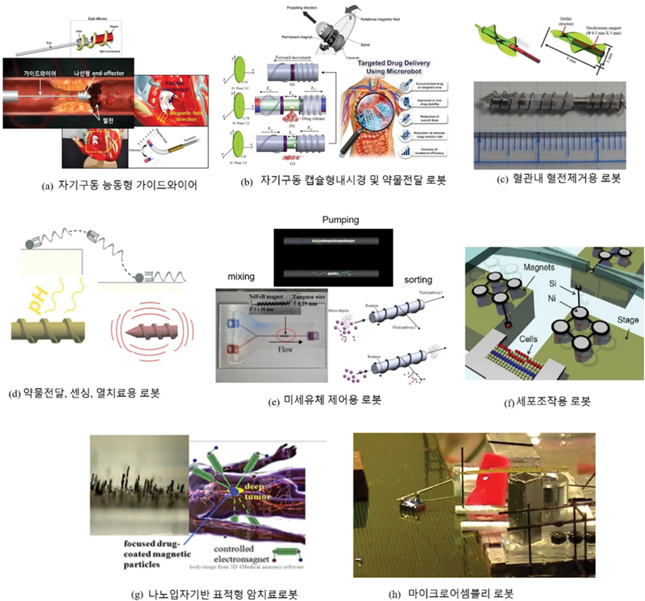
Fig. 5. (Color online) Application examples of magnetic micro/nano robot: (a) Active guidewire system [29,30], (b) Capsule-type endoscope with drug delivery robot [20,31], (c) drilling robot in blood vessel [6,10], (d) spiral-type microrobot for drug delivery and hyperthermia [15], (e) spiral-type microrobot for micro-fluid control system [4], (f) microrobot for cell manipulation [32], (g) manipulation of magnetic nanoparticles for magnetic hyperthermia [11], and (h) application of micro-assembly [1].
