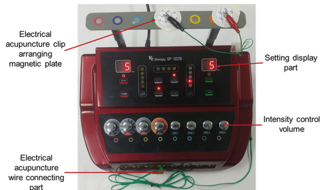
Fig. 2. (Color online) Photo of low frequency acupuncture electrical stimulator (AES) composed setting display part, intensity control volume, connecting wire part, and clip arranging magnetic plate.
