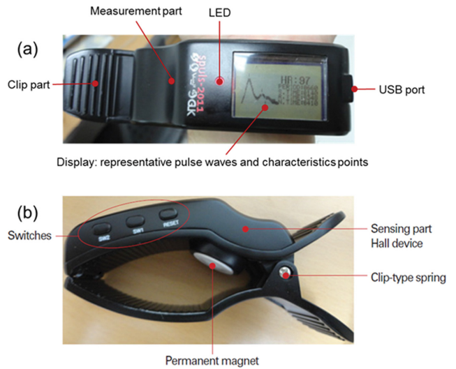
Fig. 1. (Color online) (a) Photo of pulsometer (model spuls-2011) composed of clip part, measurement part, LED, USB part, and display of representative pulse waves and characteristic points. (b) Photo of pulsometer equipped with sensing part Hall device, clip-type spring, permanent magnet, and switches.
