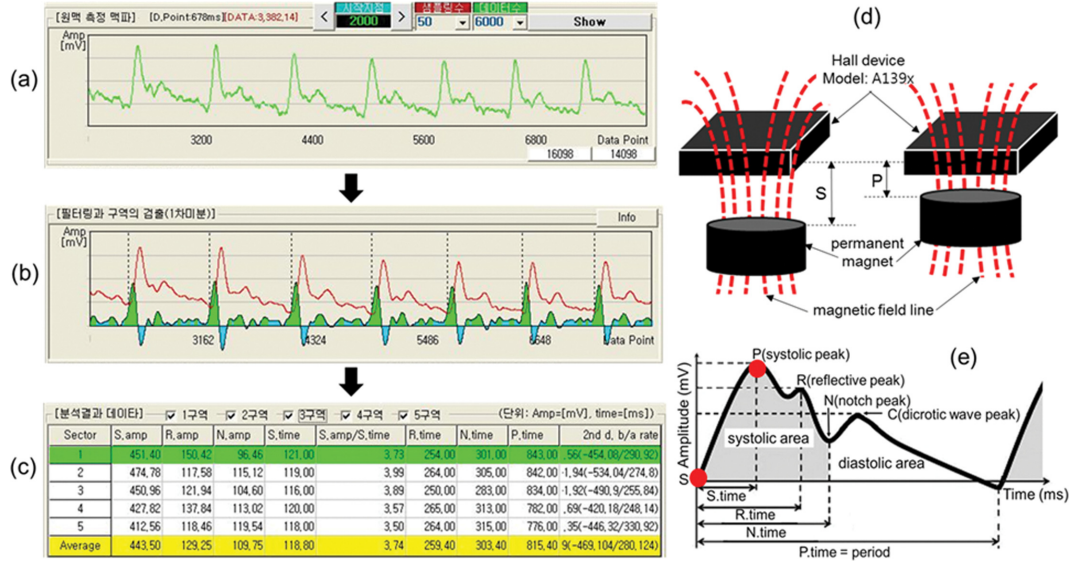
Fig. 4. (Color online) (a) Raw data, (b) filtering data, and (c) analysis table for the pulse wave measured by using the clip-type pulsimeter. The S.time obtained by the first, second, third differential methods for the average values of five continuous pulse waveforms. (d) The schematic of measuring principle of radial artery's pulse depending on a distance between Hall device and permanent magnet. (e) The output amplitudes (mV) and time (ms) corresponding to a starting point and a systolic peak point with a minimum amplitude and a maximum amplitude, respectively.
