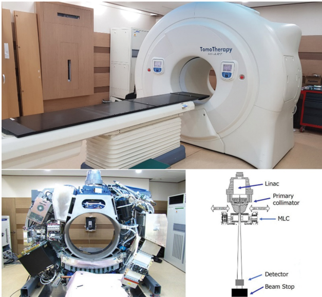
Fig. 9. (Color online) Photograph of Tomotherapy Hi-art system and schematic diagram of the Tomotherapy unit.
