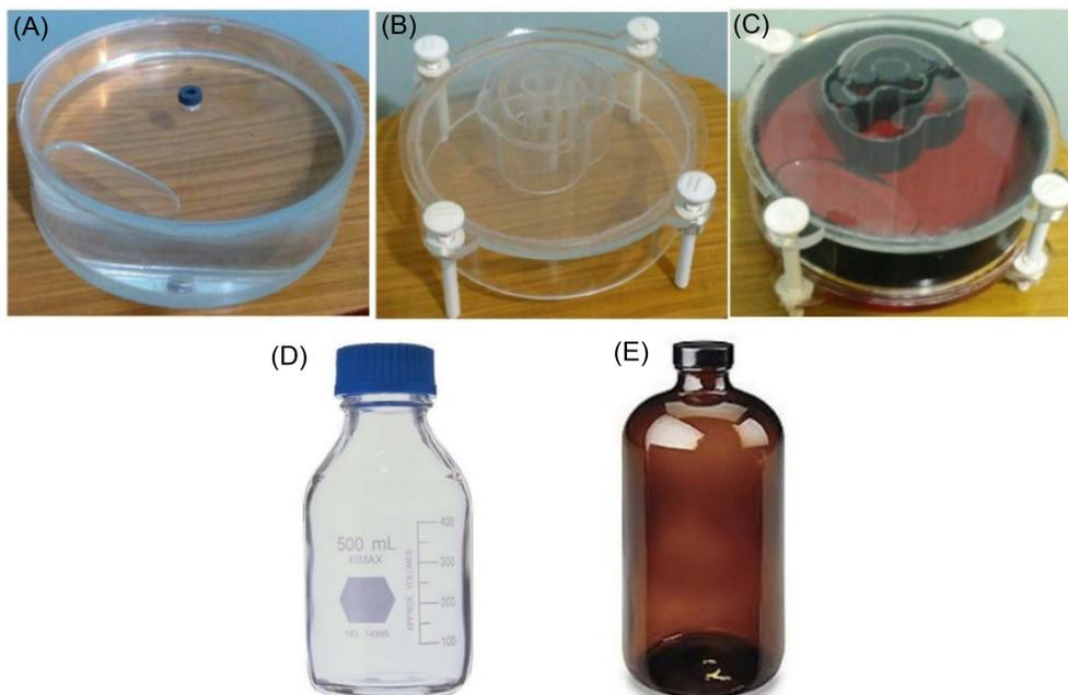
**Fig. 1.** (Color online) The phantom materials with and without internal design used to evaluate the effect of phantom material and design. (A) Homogenous Plexiglass cylindrical phantom without internal structure, (B) Plexiglass cylindrical phantom with internal structure, (C) PVC cylindrical phantom with internal structure, (D) clear laboratory glass bottle, (E) Amber laboratory glass bottle.
