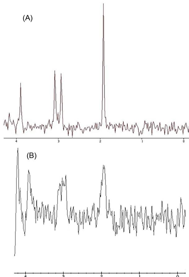
**Fig. 2.** (Color online) Spectrum of Falcon tube phantom provided by (A) 3T MR scanner and (B) 1.5 T MR scanner.
