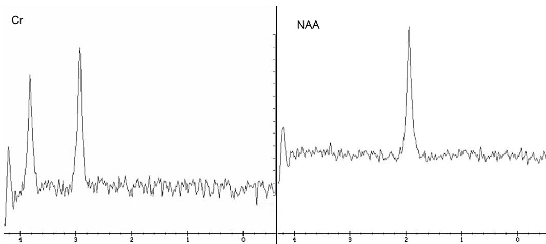
**Fig. 9.** MRS spectra of NAA and Cr using 1.5 T MRI machine, the pulse sequence of PRESS and TE of 144 ms.
