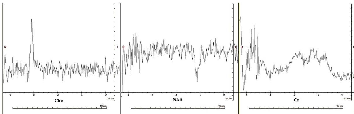
**Fig. 6.** MRS spectra of Cho, NAA, and Cr using 1.5 T MRI machine, the pulse sequence of PRESS and TE of 144 ms.
