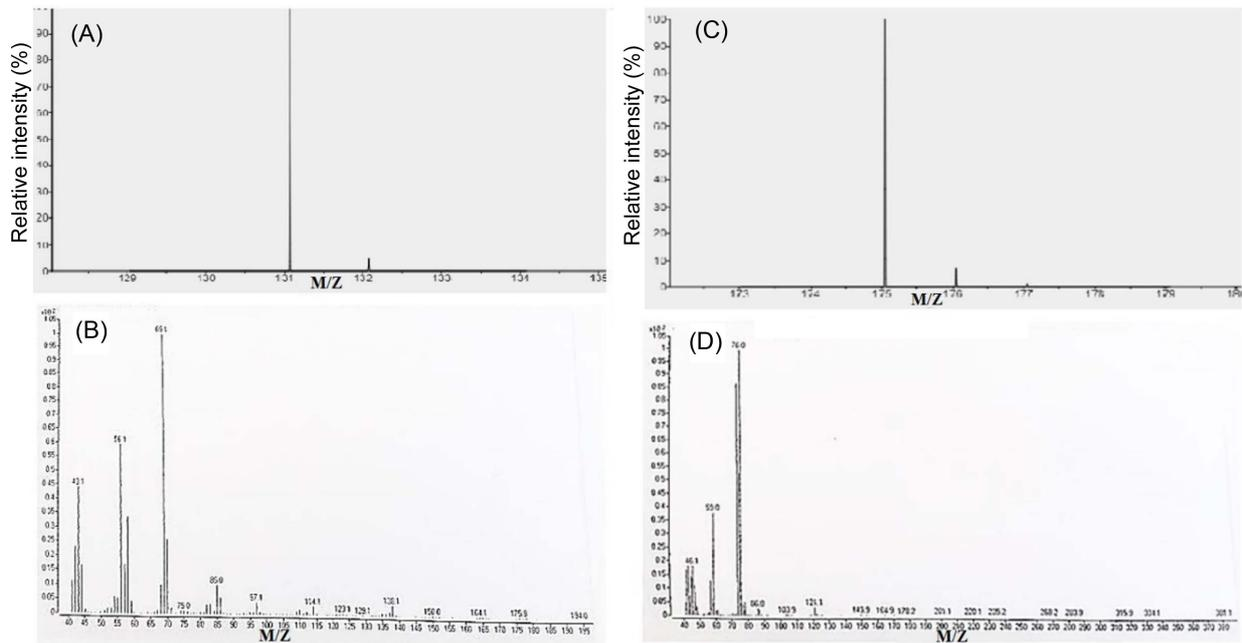
**Fig. 7.** (A) The expected result of Cr mass spectrometry. (B) The Results of the mass spectrometry of Cr. (C) The expected result of NAA mass spectrometry. (D) The Results of the mass spectrometry of NAA.
