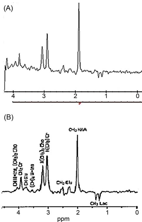
**Fig. 3.** (A) GE standard phantom spectrum. (B) the expected spectrum predicted by AAPM #9. The MRS parameters were PRESS pulse sequence, TE of 144 ms, TR of 1500 ms and voxel size of 8 cm<sup>3</sup>.
